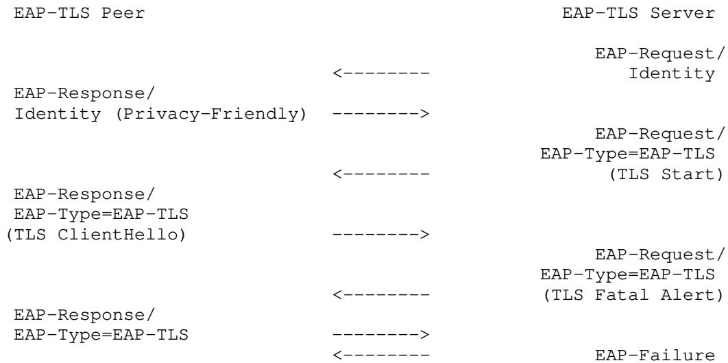
Figure 4: EAP-TLS server rejection of ClientHello
