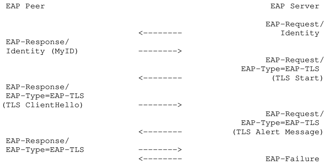
Figure 4: EAP-TLS server rejection of ClientHello
