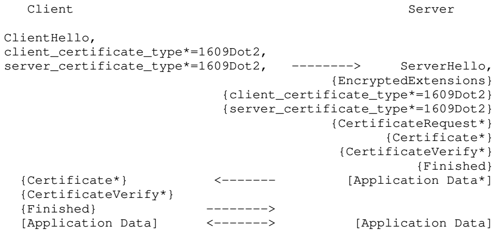
Figure 2: TLS Client and TLS Server use the IEEE 1609.2 certificate
