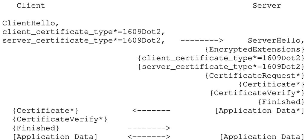
Figure 2: TLS Client and TLS Server use the IEEE 1609.2 certificate
