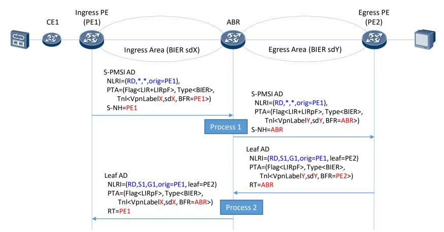
Process 1: per-vpn info: FEC=(RD,PE1), upstream (X, PE1), downstream(Y, ABR) Process 2: per-flow info: FEC=(RD,PE1,S1,G1), upstream(X,PE1), downstream(Y,ABR,PE2)
