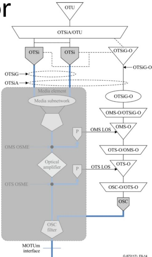
Figure 8-14 – Example of a terminal implementation using a single media element
