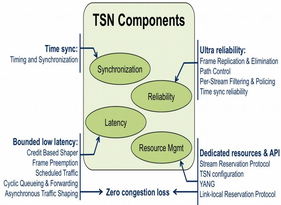
Time Sensitive Networking is an enhancement to IEEE 802 networks enabling the convergence of real-time control with time-critical streaming and and bulk data into a single communication network.
