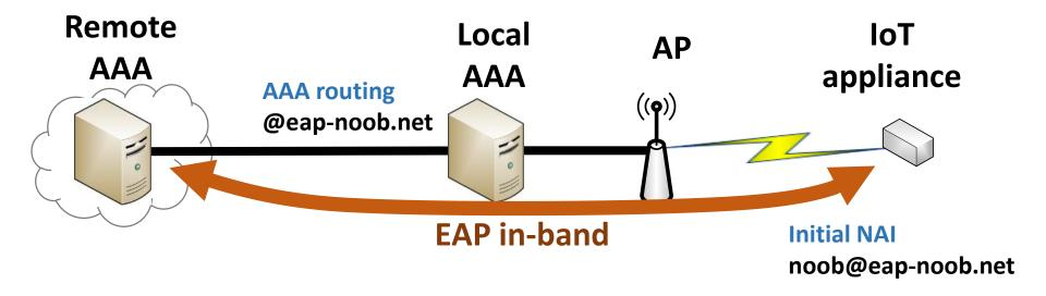
EAP tunnel and AAA routing enable in-band communication with the authentication server *before* the device is registered
