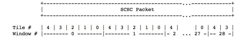
Figure 9: a SCHC Packet fragmented in tiles grouped in 28 windows, with WINDOW SIZE = 5
