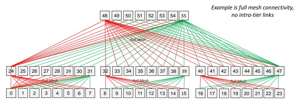
The blueprint for the flooding topology is two diversely rooted spanning trees. In the illustrated example they are nodes 0 for the red and 55 for the green trees. The red spanning tree was constructed with algorithm mask 0
