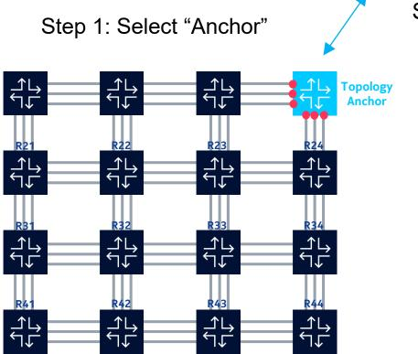
Step 2: Adj router to Clamp to "Anchor" (using RPF info towards "Anchor")
