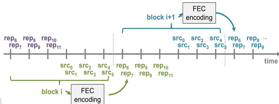
two output leaky buckets: repair and source packets transmitted in parallel
