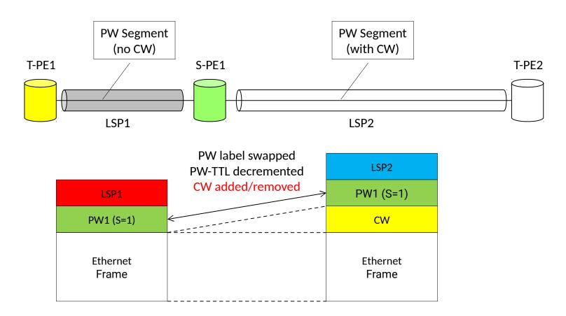
No changes are required in T-PE1 and T-PE2 nor in intermediate P nodes
