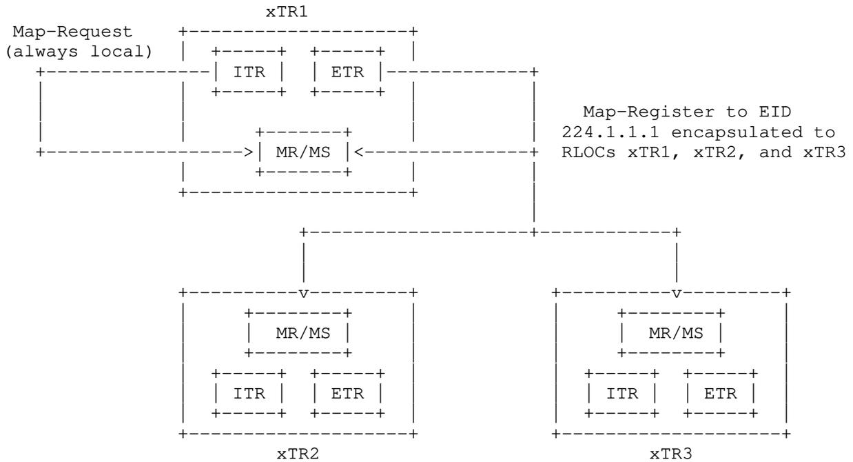
Note if any external xTR would like to use a Map-Resolver from the mapping system group, it only needs to have one of the LISP-Decent Map-Resolvers configured. By doing a looking to this Map-Resolver for EID 224.1.1.1, the external xTR could get the complete list of members for the mapping system group.
