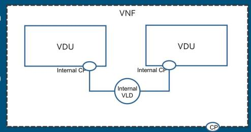
• The VDUs attach to the internal VLs using the internal Connection Points (CPs).
