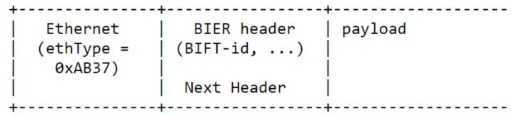
BIER-ETH encap (BIER header for Non-MPLS networks as defined in [RFC8296]) can be used to transport the multicast data in the IPv6 network by encapsulating the multicast user data payload within the BIER-ETH header. However, using BIER-ETH in IPv6 networks is not considered to be a native IPv6 solution which utilizes the IPv6 header to forward the packet.
