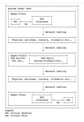
Figure 5 NVE Split not collocated - System Under Test
