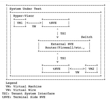
Figure 4 NVE Split collocated - System Under Test
