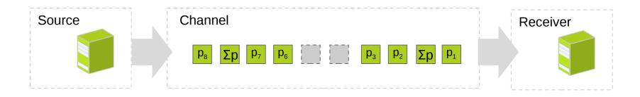
Using coded packets long delays can be avoided. In the above example the receiver is able to recover from the two packet losses when receiving the second coded packet.
