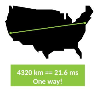
The distance from Stanford to Boston is ~4320km. The speed of light in vacuum is 300 x 10<sup>6</sup> m/s. The speed of light in fibre is roughly 66% of the speed of light in vacuum. The speed of light in fibre is  $300 \times 10^6 \text{ m/s} \times 0.66 = 200 \times 10^6 \text{ m/s}.$ The one-way delay to Boston is  $4320 \text{ km} / 200 \times 10^6 \text{ m/s} = 21.6\text{ms}.$
