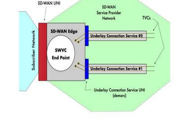
Figure 1 - Components of an SD-WAN Service
