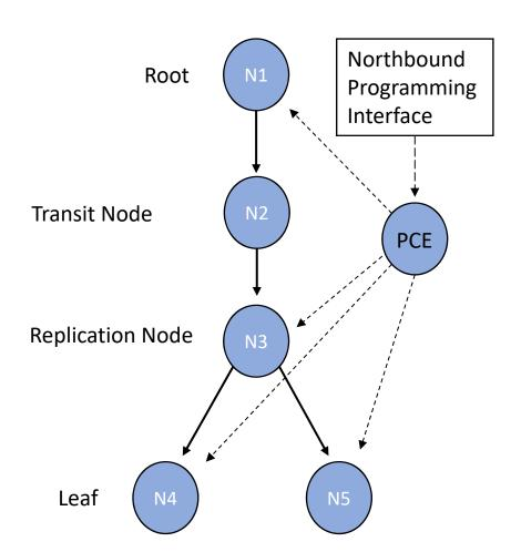
A SR Replication policy can be instantiated and maintained in a centralized fashion using a Path Computation Element (PCE)
