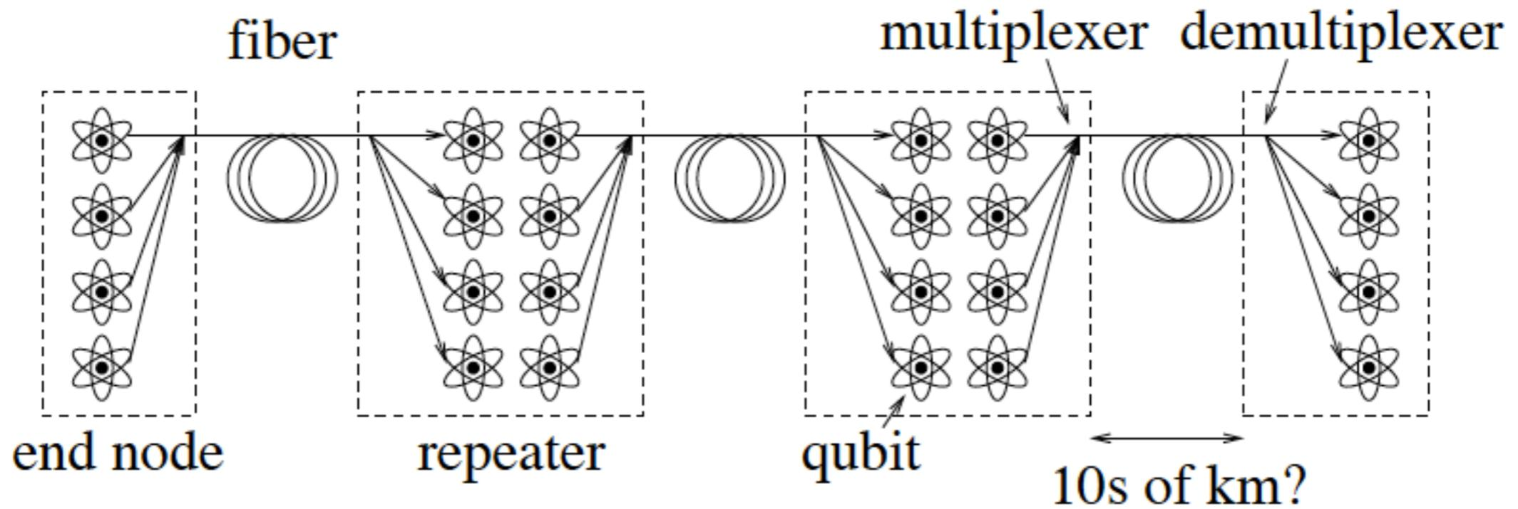
Figure 10.1: Generic view of the hardware of a line of repeaters. Qubit memories are represented by the atom symbol, regardless of physical device type.
