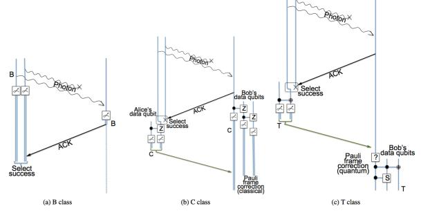
FIG. 2: Timing for application classes over a single forward-propagating link.
