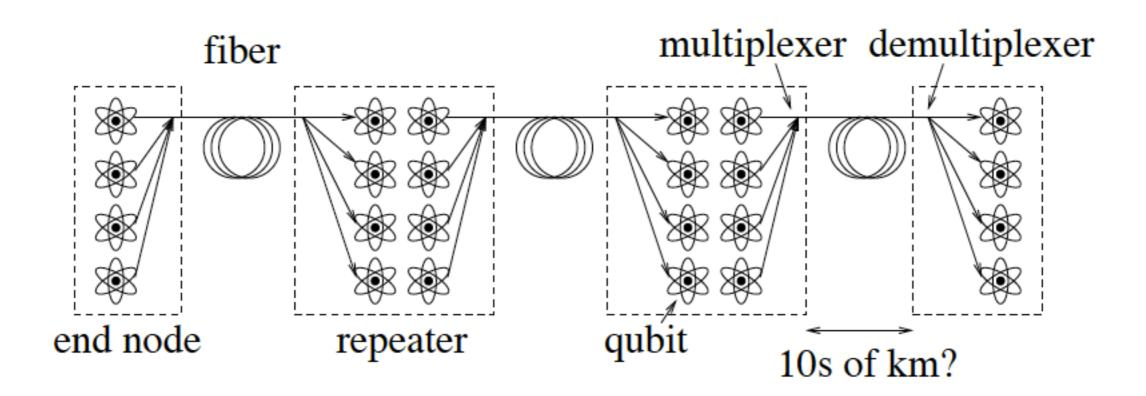
Figure 10.1: Generic view of the hardware of a line of repeaters. Qubit memories are represented by the atom symbol, regardless of physical device type.
