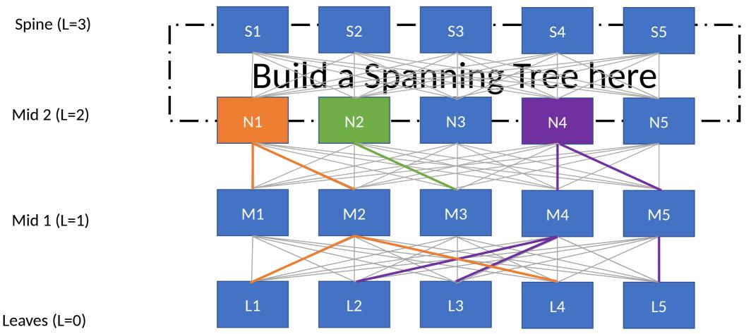
The spanning tree must span all subToF and may span some or optionally all ToF nodes
