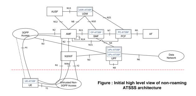
Mobile device multi-connectivity based on expected 3GPP Rel. 16 ATSSS specification
