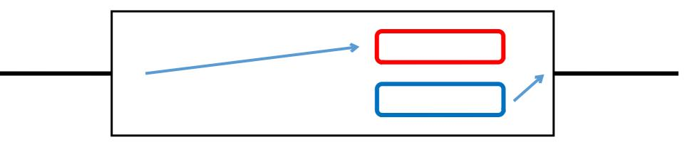
• Two-buffer version: Two buffers per port. Input and output buffers swap at the same moment, once every cycle, period  $T_c$ . Small guard band to allow for transit and forwarding time. All relay nodes are synchronized and swap buffers at the same moment. Cycle time  $T_c$  > transit time + forwarding time + clock inaccuracy + max data transmit time.
