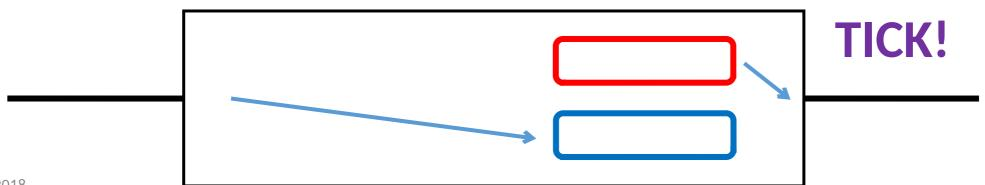
• Two-buffer version: Two buffers per port. Input and output buffers swap at the same moment, once every cycle, period  $T_c$ . Small guard band to allow for transit and forwarding time. All relay nodes are synchronized and swap buffers at the same moment. Cycle time  $T_c$  > transit time + forwarding time + clock inaccuracy + max data transmit time.
