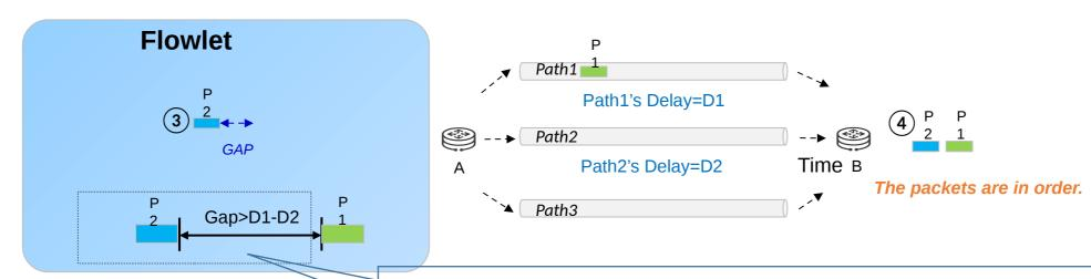
Allocating P2 a high-priority queue in the router, to avoid queuing time; and finding P2 a proper queue which has a queuing time larger than the gap time.
