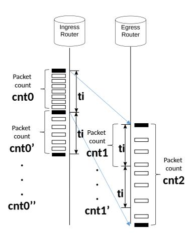
The Egress router read the cnt1 every ti interval, and send the result to the ingress; the Ingress gathers the results, and do calculation in everty ti\*N interval. (e.g., ti=3.3ms, N=3)
