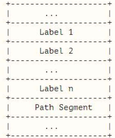
Figure 1: Label Stack with Path Segment
