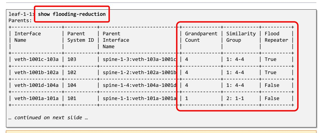
Provides details needed to understand the outcome of the flood repeater election algorithm.
