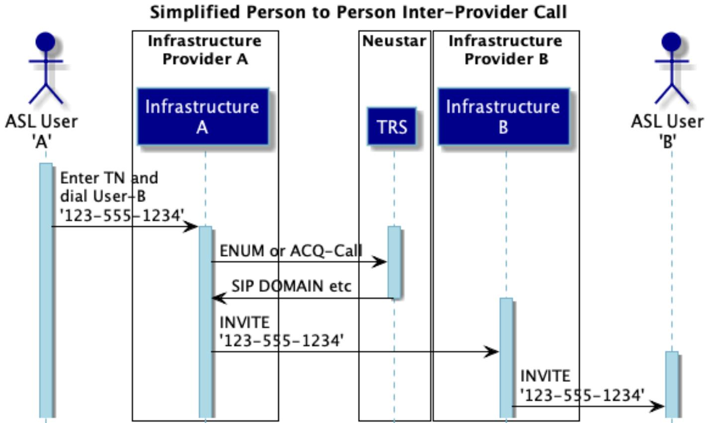
Note: Sequence diagram is indicative only. It does not reflect the full call flow.
