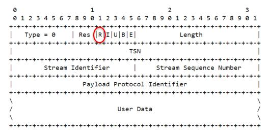
Figure 1: Extended DATA chunk
