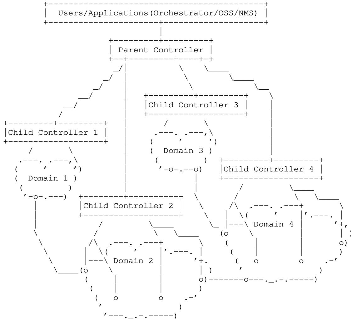
The parent controller communicates with these four child controllers and controls them, each of which controls (or is responsible for) a domain. Child controller 1 controls domain 1, Child controller 2 controls domain 2, Child controller 3 controls domain 3, and Child controller 4 controls domain 4.
