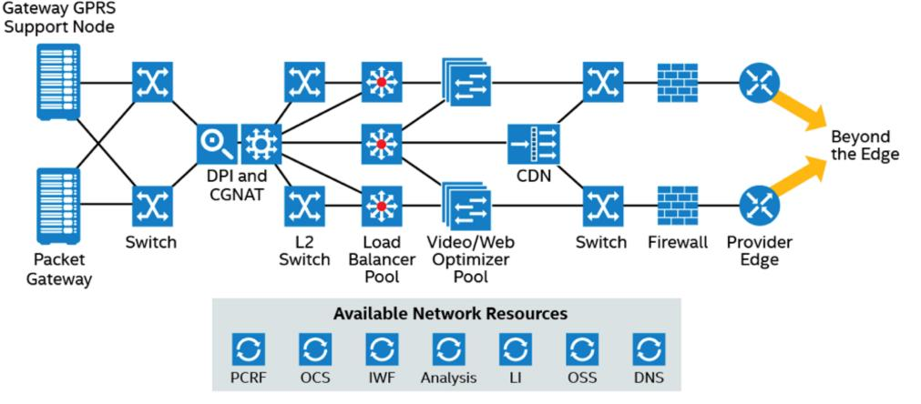
CDN – content delivery network; CGNAT – Steering/Carrier Grade Network Address Translation; DPI – deep packet inspection; DNS – domain name system; GPRS – General Packet Radio Service; IWF – interworking function; LI – lawful interception; OCS – online charging system; OSS – operational support system; PCRF – policy and charging rules function
