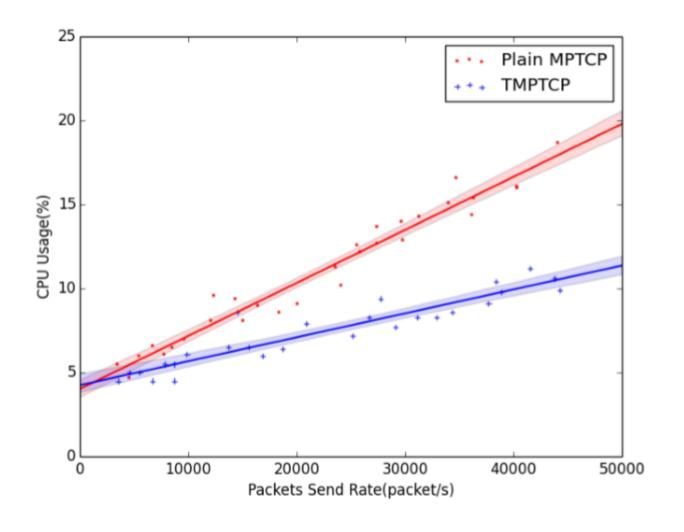
Fig. 6. CPU Usage Comparison between Plain MPTCP and TMPTCP
