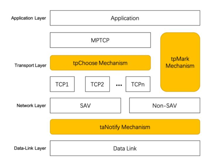
Fig. 1. TMPTCP Framework: three extended mechanisms on the network protocol stack
