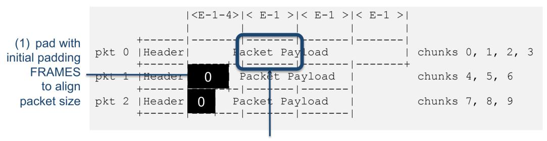
(2) segment padded payloads into E-1 byte long chunks (E-5 for the 1<sup>st</sup> one to leave room for additional info)
