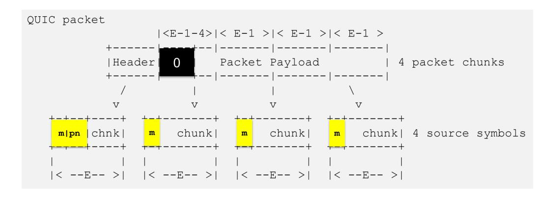
• to be used for FEC encoding/decoding, not transmitted per se
