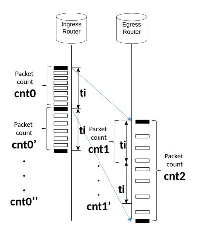
The Egress router read the cnt1 every ti interval, and send the result to the ingress; the Ingress gathers the results, and do calculation in everty ti\*N interval. (e.g., ti=3.3ms, N=3)
