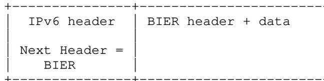
Between two directly connected BFRs, a BIER header can directly follow link layer header, e.g., an Ethernet header (with the Ethertype set to 0xAB37). Optionally, IPv6 encapsulation can be used even between directly connected BFRs (i.e. one-hop IPv6 tunneling) in the following two cases:
