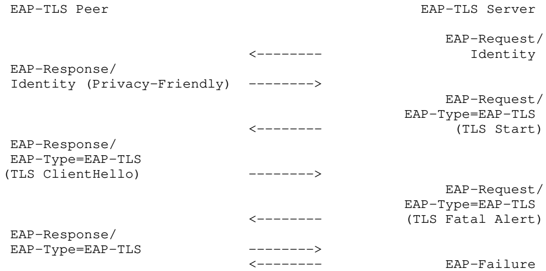
Figure 5: EAP-TLS server rejection of ClientHello
