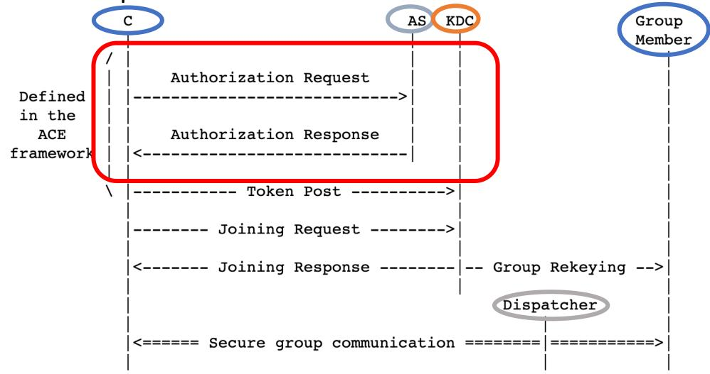
Figure 2: Message Flow Upon New Node's Joining
