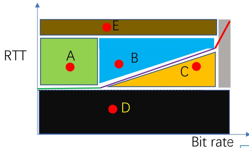
Cloud Gaming APP is sensitive to the latency and bandwidth. The Cloud Gaming APP needs to detect the network capability, determines its status (as the left figure) and changes its APP functions or codec scheme.
