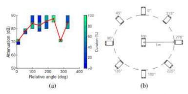
Fig. 4: (a) Measured attenuation duration vs the angle between two handsets placed 1m apart. (b) Schematic showing orientation to which each angle corresponds.
