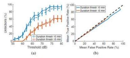
Fig. 8: Exposure notification true and false positive rates when a simple threshold strategy is applied to the GAEN tram dataset. (a) True and false positive rates vs attenuation level and duration thresholds, solid lines indicate true positive rates and dashed lines the corresponding false negative rates. (b) ROC plot corresponding to mean rates in (a), dashed line indicates  $45^{\circ}$  line.
