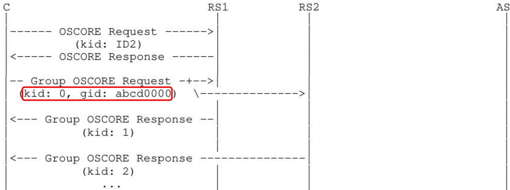
**C can access RS1 and RS2 resources, as per the posted Access Token, using OSCORE or Group OSCORE**
