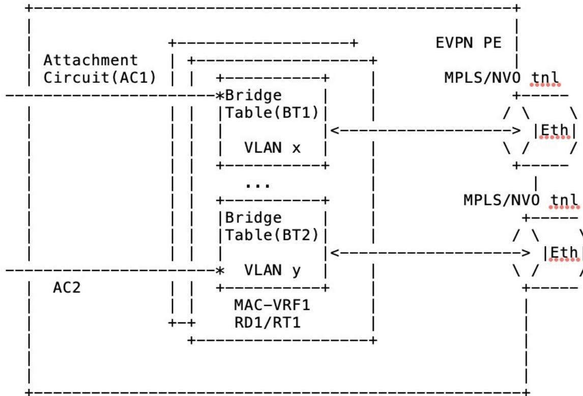
Figure 1: EVPN IRB PE Model
