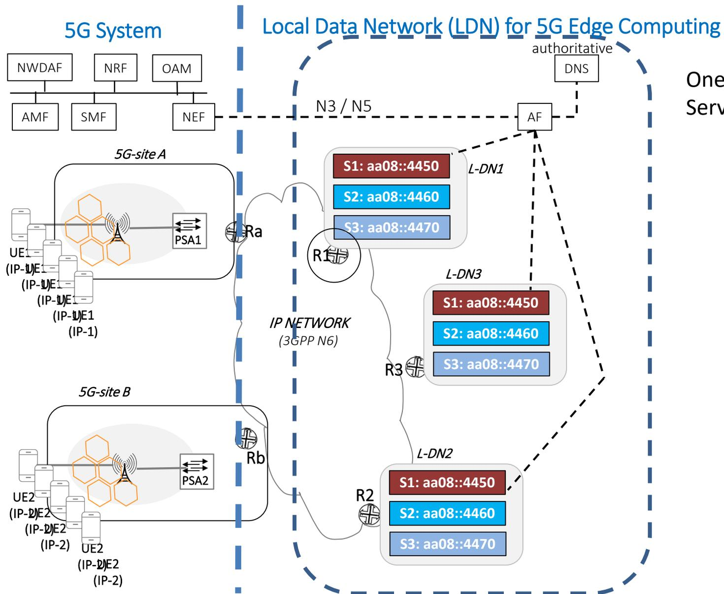
One Application has multiple Application Servers located in Edge Computing DCs
