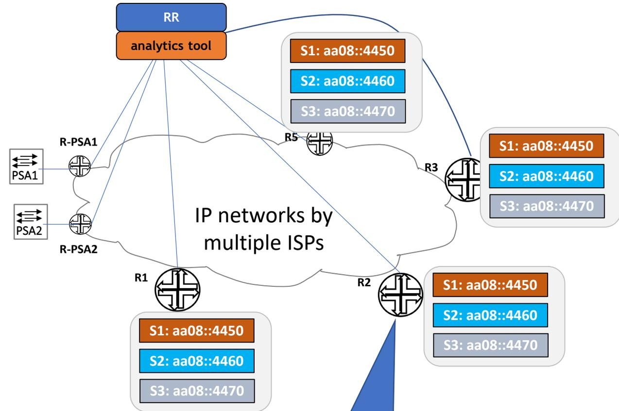
BGP UPDATE for its attached App Server ANYCAST address include: Load Index, Capacity Index, and Site Preference
