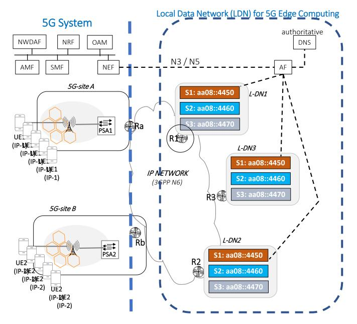
One Application has multiple Application Servers located in Edge Computing DCs
