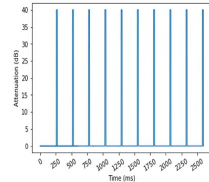
Figure 3: Attenuation over time to simulate a DVB Satellite - Mobile receptor link
