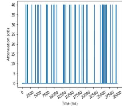
Figure 2: Attenuation over time to simulate an Optical Satellite link
