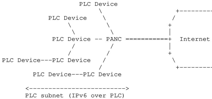
Figure 6: PLC Tree Network connected to the Internet
