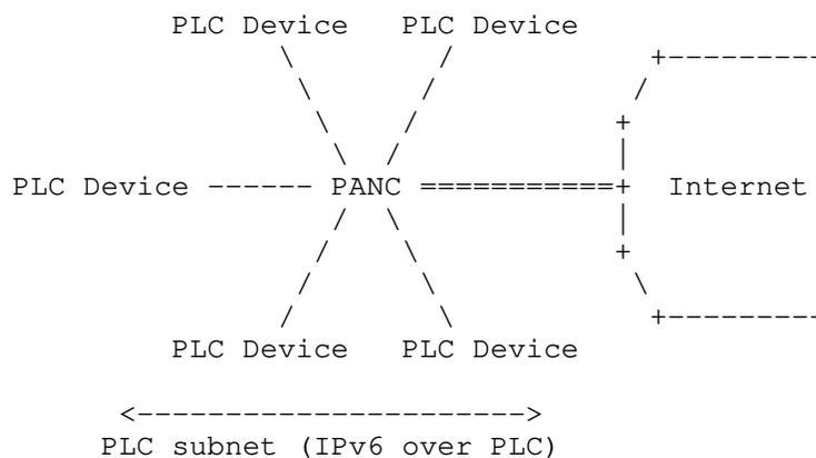
Figure 5: PLC Star Network connected to the Internet
