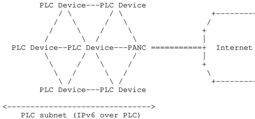
Figure 7: PLC Mesh Network connected to the Internet
