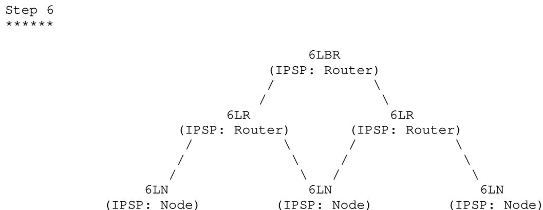
Figure 3: An example of connection establishment and use of IPSP roles in an IPv6 mesh over Bluetooth LE links.
