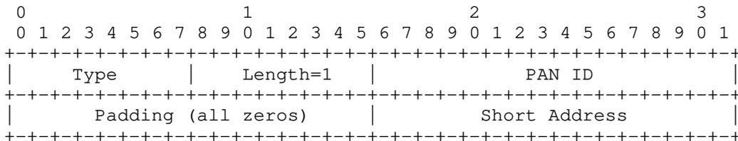
Figure 4: Unicast Address Mapping for IEEE 1901.2
