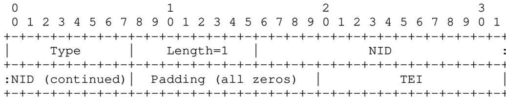
Figure 3: Unicast Address Mapping for IEEE 1901.1
