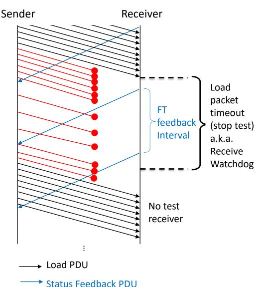
**Operation:** The load packet timeout SHALL be reset to the configured value each time a load packet received. If the timeout expires, the receiver SHALL be closed and no further feedback sent.
