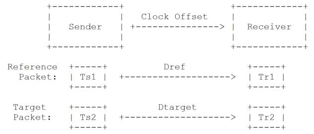
Figure 2: Topology of One-way Delay Measurement
