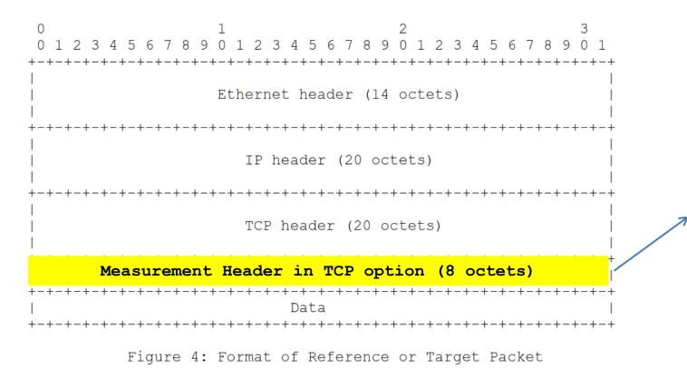
The sender encapsulates timestamp information and sender-receiver pair information in the Measurement Header of the sent packet.
