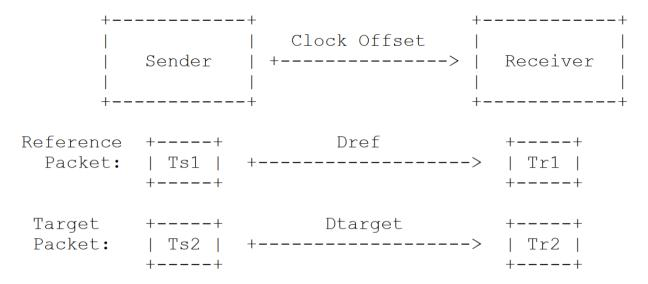
Figure 2: Topology of One-way Delay Measurement
