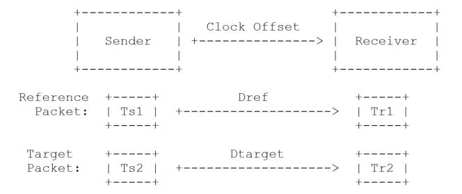
Figure 2: Topology of One-way Delay Measurement
