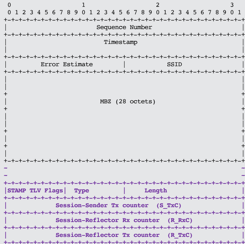
Figure: STAMP Session-Sender Test Packet Format
