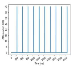
Figure 3: Attenuation over time to simulate a DVB Satellite - Mobile receptor link
