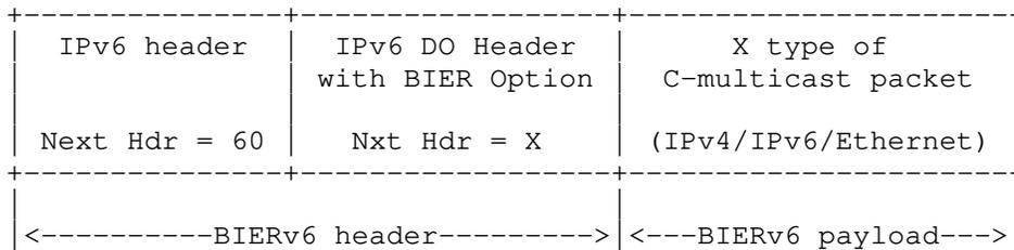
BIERv6 proposes to define a new type of destination options header for BIER. The destination address of the IPv6 header indicates the BIER forwarding nodes and changed to the next BIER forwarding nodes based on the result of BIER forwarding table lookup.
