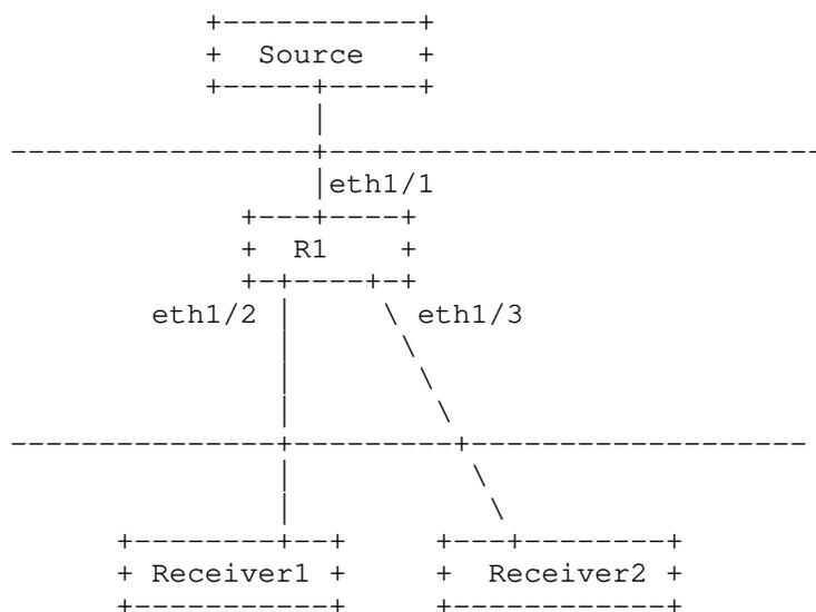
The configuration data for R1 in the above figure could be as follows:
