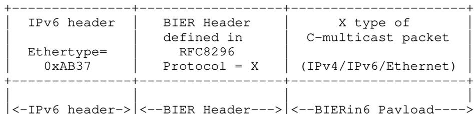
BIERin6 proposes to encapsulate the IPv6 header before the BIER header in order to transit the BIER header through IPv6 nodes by adding IPv6 header between BIER forwarding nodes. The "next header" codepoint of the IPv6 header is set to the value that means that "the next header is non-MPLS BIER".
